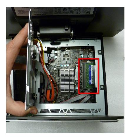
5. Using fingers push the RAM retainer clips outward to release the RAM module. The RAM will spring upward when fully released.
