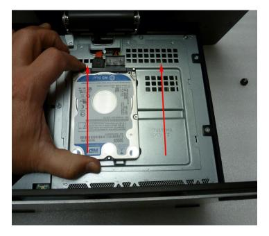
4. Lift front metal plate away from unit to gain access to the RAM module.
