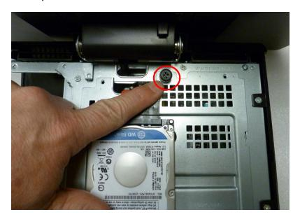
3. Grasp the HardDrive and push in upward direction to release the front metal plate of unit.
